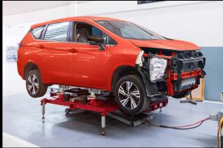
Your vehicle's frame may become misaligned after an accident. With our expert techniques and skills, we accurately measure and effectively correct any frame damage, restoring your car's structural integrity for optimal safety.
